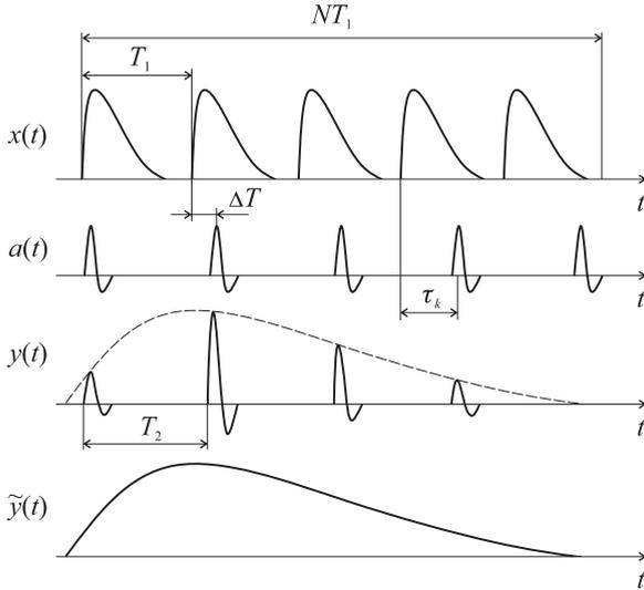
Fig. 3. The stroboscopic transformation of the timescale of periodic signals.
