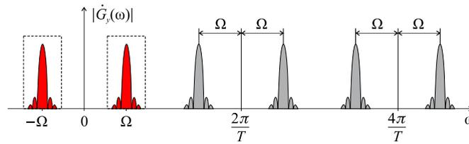
**Fig. 4.** The spectrum  $|\hat{G}_y(\omega)|$  of the signal  $y(t)$  on return of the stroboscopic mixer for  $\Omega < \pi/T$ . Red color denotes the filtered spectral components. (For interpretation of the references to color in this figure caption, the reader is referred to the web version of this paper.)
