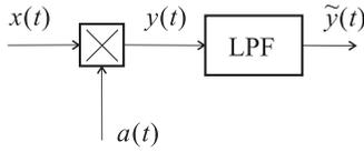
Fig. 2. The mathematical model of the stroboscopic transformer of the timescale.
